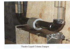
Tsuboi Liquid Column Damper
