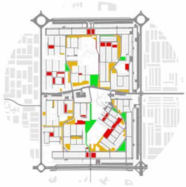
Figure 3: plan of sector 22, Chandigarh, showing categories of open spaces Green: Active, Yellow: Auxiliary, Red: Non-active (Source : Author, 2020)
