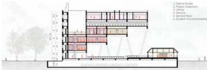
Fig 3.4(a): Section - Shaded plazas created on the ground level to allow interaction (Source: Author).
