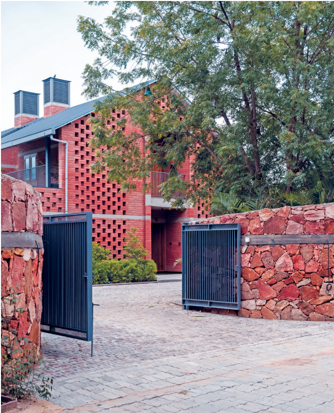
External view of the Jalmanjar Farmhouse on the outskirts of Ahmedabad. The jaali wall is meant to cool the house down as it acts as an external skin.
