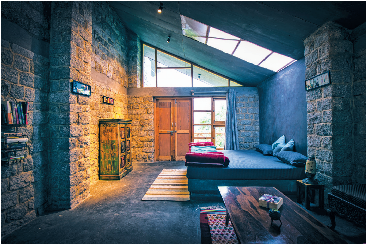
One of the rooms at Someplace, Manali, showcasing larger windows towards the south for maximum heat gain.
