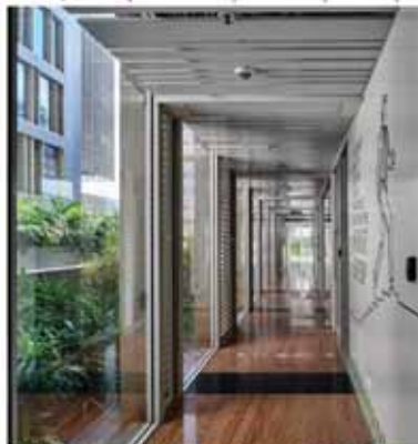
Circulation areas of the tower blocks are cooled using natural ventilation only
