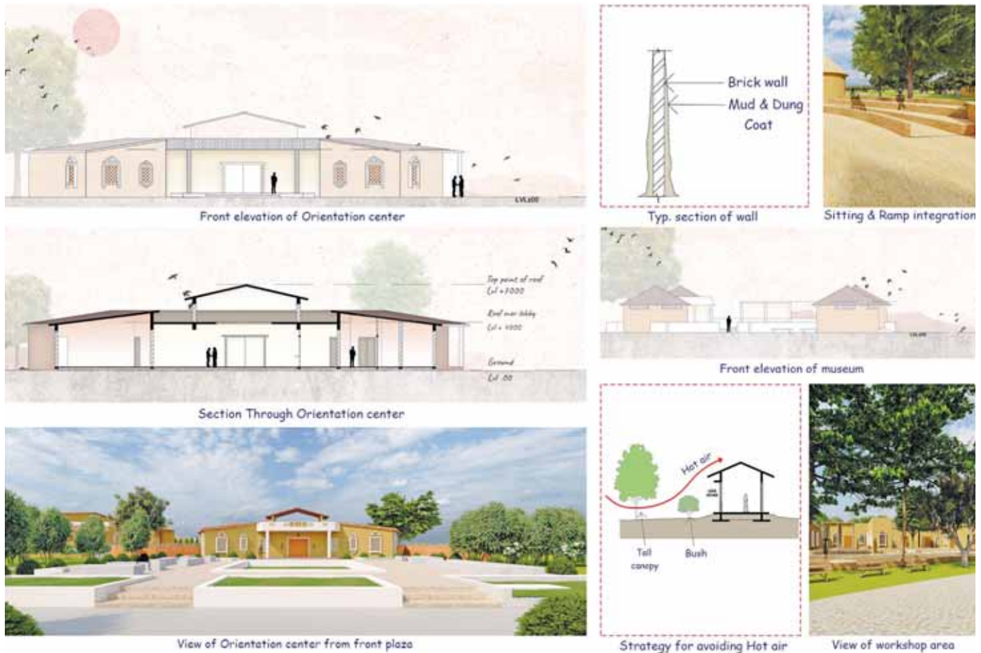
Figure 6: Elevation and strategies to avoid harsh climate Source: Authors
