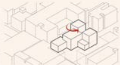
Each function of the house were identified as individual volumes and then introduced to a game of twisting, stacking and interlocking creating curious spaces and angles.
