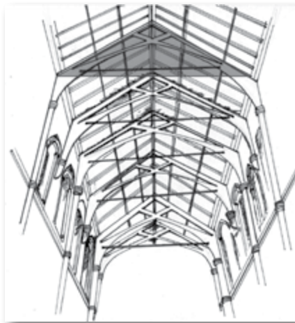
6. Scissor Braced roof truss, Source: Author
