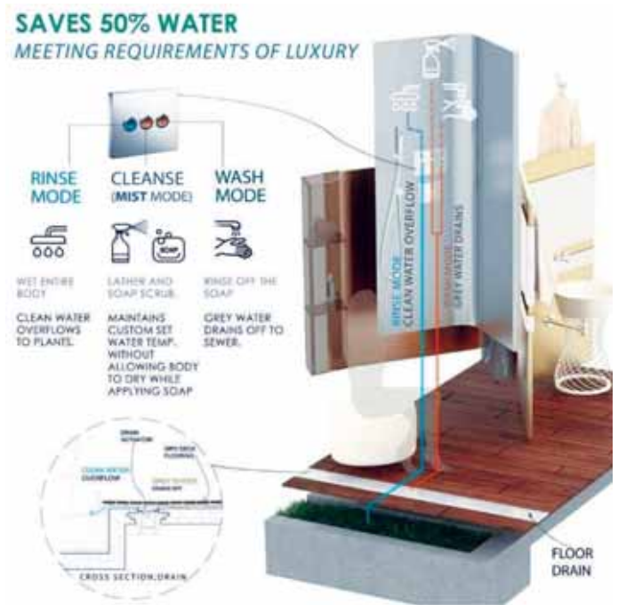
Figure 1: Illustrates a perspective view of multi-mode shower according to the present invention
