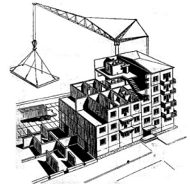
A large-panel concrete building under construction
