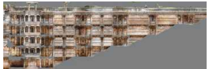
Figure 1: Orthomosaic generated through photogrammetry of Bai Harir ni Vav Stepwell, Ahmedabad
