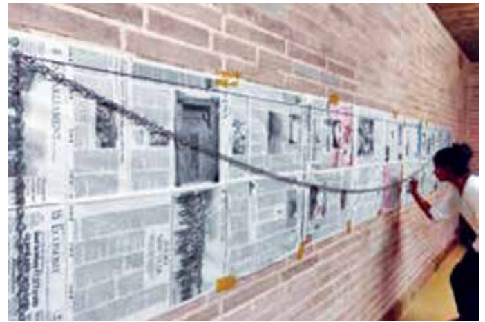
Fig 8: A catenary arch with our design span (4.47m) & rise (447mm) was traced from a hanging chain Source: Kakani Associates
