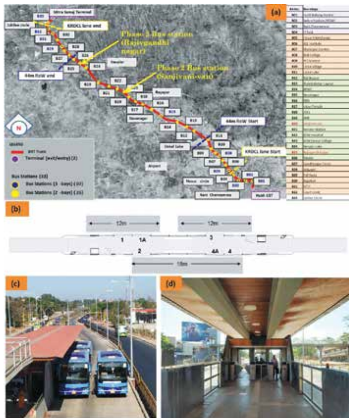
Figure 6: (a) HDBRTS corridor with BRT stations location (b) Bus station design for 18m long articulated buses; (c) Bus station with BRT Buses; (d) Bus station Interiors
