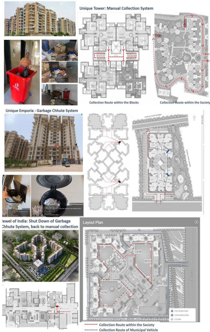
Figure 8: Waste collection and Transfer process – Unique Tower (Top), Unique Emporia (Middle) and Jewel of India (Bottom) respectively Source: Author
