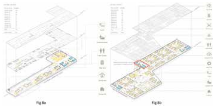
Figure 8: Site arrangements - a: Narrow site with G+1 clusters, b: Spread-out site with single storey clusters
