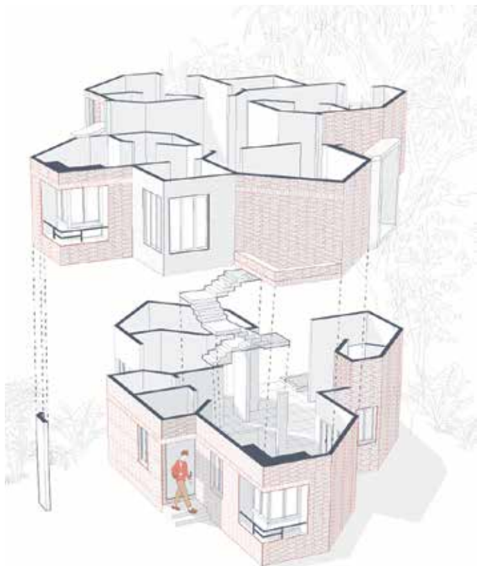
Image 3: An exploded view of the Karna Bungalow reveals its key elements: central staircase, gradually rising levels and chamfered corners. Illustration credits: Aejaz Sheikh
